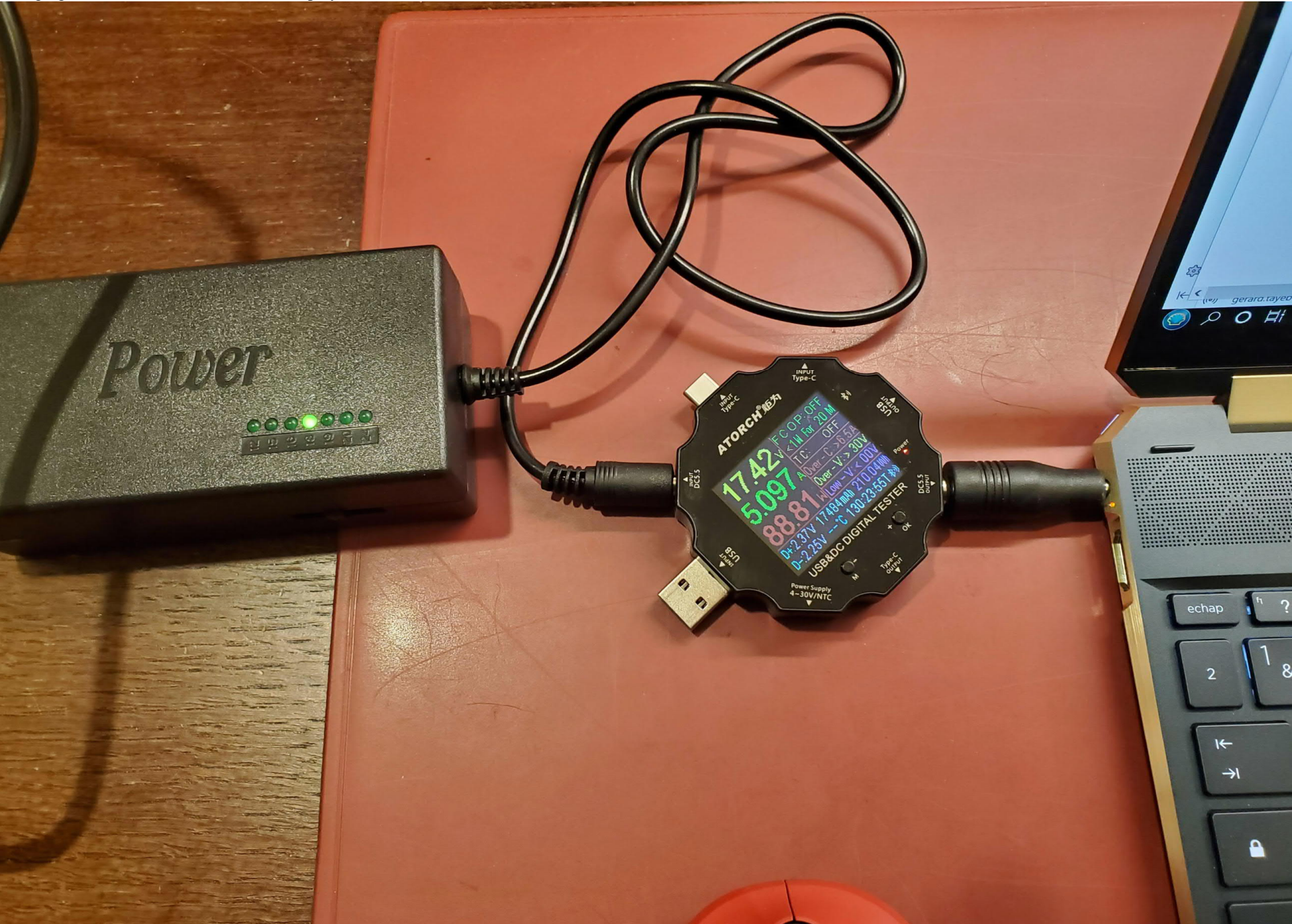
Charging at 18V . in that case the tester displays 17.42V, 5.097A, and 88.81W
