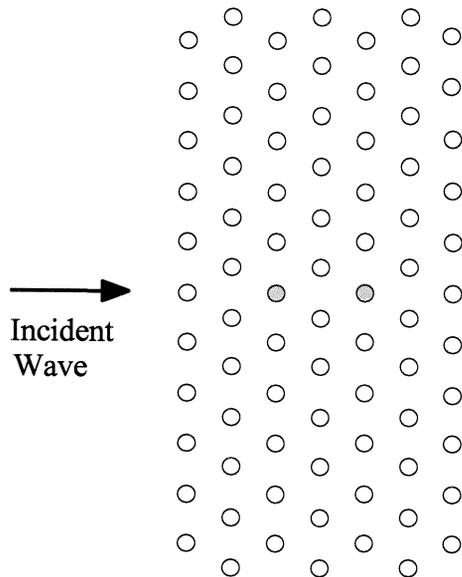
Fig. 1. Scheme of the photonic crystal. In the non-doped crystal, all the rods are present. The doped crystal is obtained by suppressing the two grey rods.
