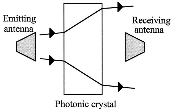
Fig. 7. Transmission through the crystal according to the ultrarefraction conjecture.
