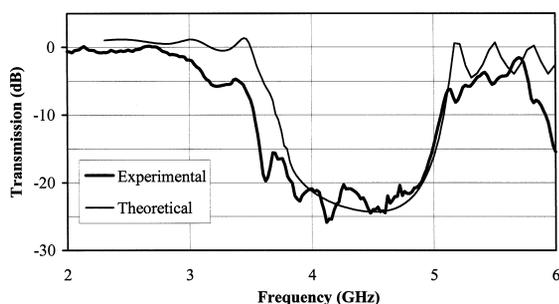
Fig. 4. Transmission curves for the non-doped crystal.
