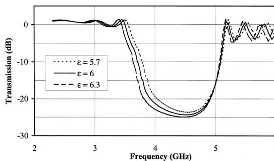
Fig. 6. Non-doped crystal: theoretical results for different values of the permittivity  $\epsilon$ .
