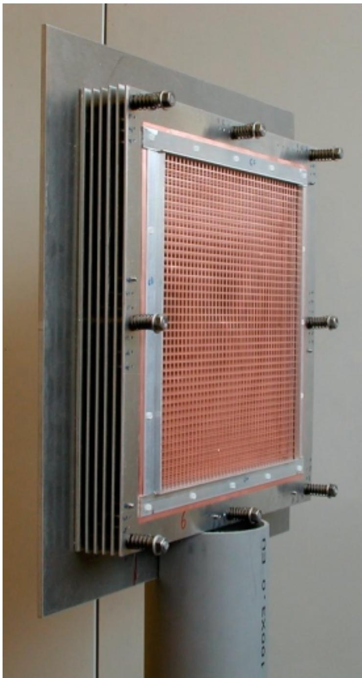
Antenna with 6 grids etched from copper sheets
