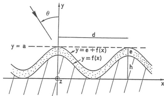
Figure 3. A particular case of fig.2 : a coated grating
