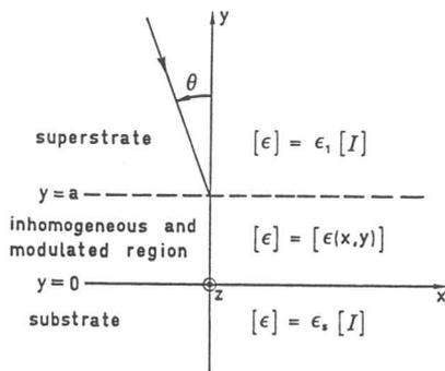
Figure 2. The structure we study in the differential method. The region  $y < a$  may be filled with lossy materials
