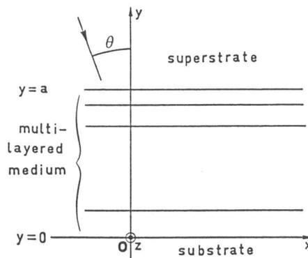
Figure 1. Multilayered media. The layers ( $0 < y < a$ ) and the substrate are made of anisotropic materials.
