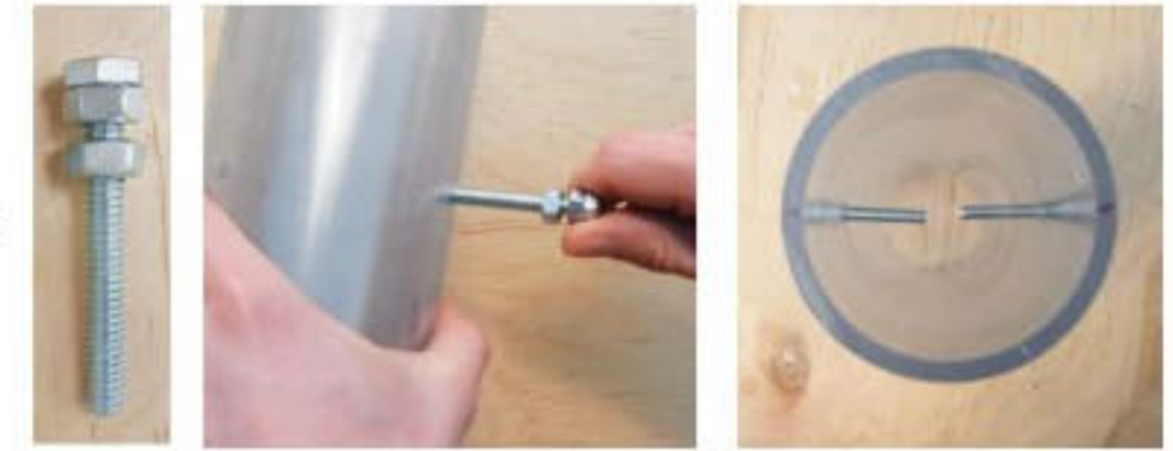
This is the spark gap that will ignite the fuel, firing the cannon.
