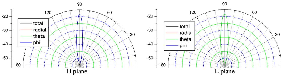
Fig.5: Radiation patterns obtained by the 3D modeling (dB scale).
