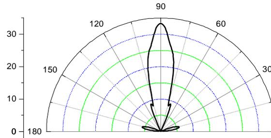
Fig.4: Radiation pattern for the device of Fig.3 (dB scale). The half-power beamwidth is  $2 \times 3.8^\circ$ .
