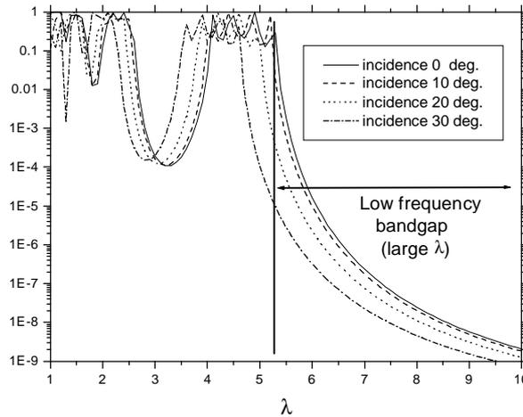
Fig.2. Transmission of a plane wave through a stack of 5 grids with  $d_x = 1$  and  $d_y = 2$ . The radius of the wires is  $r = 0.05$ . All dimensions can be scaled by multiplication by an arbitrary factor.
