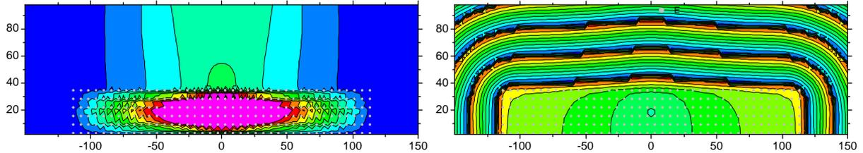
Fig. 3: Field modulus (left) and lines of equal phase (right) of the field radiated by the 2D antenna.
