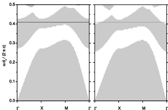
FIG. 2. Left: representation of the dispersion relation in the simple cubic photonic crystal. Right: dispersion relation in the expanded cubic photonic crystal. The gray regions are the regions where no solution exists. The black line is for  $\omega d_x / (2 \pi c) \approx 0.409$ , corresponding to  $\lambda \approx 7.83 \mu\text{m}$ .
