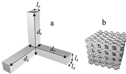
FIG. 1. a: Elementary cell of a simple cubic photonic crystal. Unexpanded photonic crystal:  $d_x=d_y=d_z=3.2 \mu\text{m}$  and  $l_x=l_y=l_z=0.8 \mu\text{m}$ . Expanded photonic crystal: same dimensions except  $d_z=3.41 \mu\text{m}$  and  $l_z=0.85 \mu\text{m}$ . The optical index of the dielectric is  $n=3.6$  and the embedding medium is vacuum. (b) Example of a  $5 \times 5 \times 5$  cell simple cubic photonic crystal.
