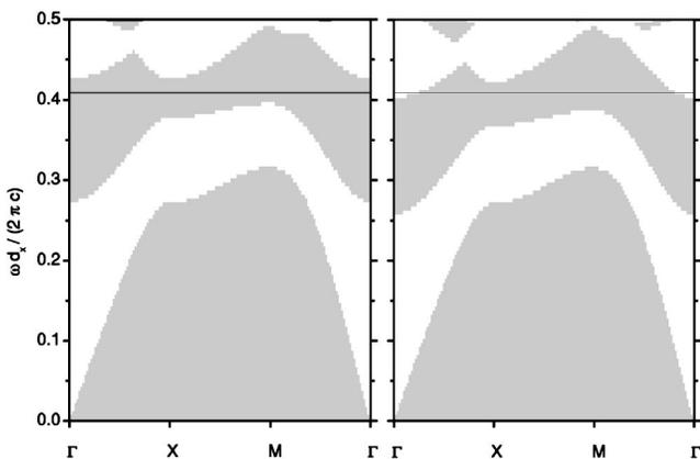
FIG. 2. Left: representation of the dispersion relation in the simple cubic photonic crystal. Right: dispersion relation in the expanded cubic photonic crystal. The gray regions are the regions where no solution exists. The black line is for  $\omega d_x / (2 \pi c) \approx 0.409$ , corresponding to  $\lambda \approx 7.83 \mu\text{m}$ .
