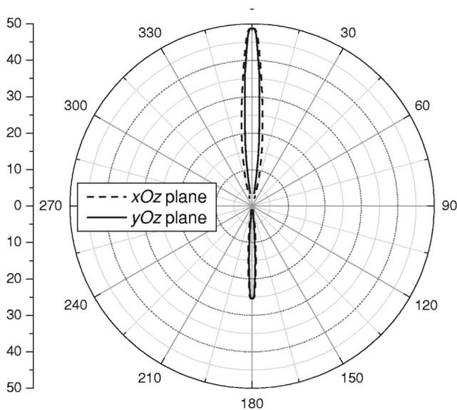
FIG. 3. Normalized emitted power in the dB scale by a dipole in the  $yOz$  (solid line) and  $xOz$  planes (dashed line). The oscillating dipole at  $\lambda = 7.83 \mu\text{m}$  is directed along  $Oy$  and located at the middle of the expanded crystal, more precisely in the center and at the top of a vertical dielectric rod between the third and fourth layers of the expanded crystal.
